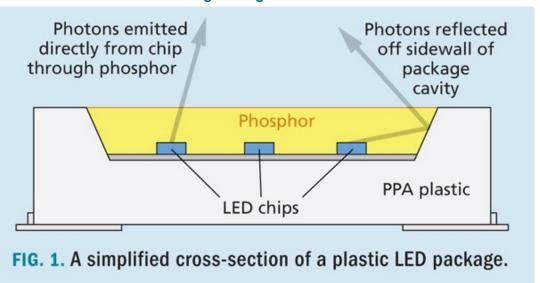
On a direct-light LED circuit board, is a grid of attached pixels – or the smallest addressable components on the display from the perspection of content delivery. These "pixels" typically are what is referred to in the industry as a "package" and as you might expect, given the name, these actually are comprised of a number of individual elements – all of which can be differentiators in the performance and efficiency of the display.
