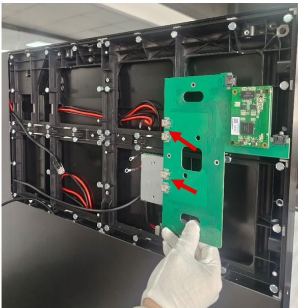
Remove the screws that secure the cable, and the HUB card can be removed
