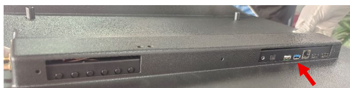
★ When removing the cover, please be careful with the USB port
