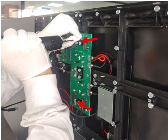
Remove the 2 screws that secure the HUB card
