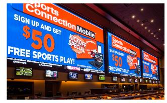
dramatically brighter than the projection video system they were replacing," observed H Waldman, Chief Operating Officer at National Technology Associates. The screens each measured 31.5-feet-wide-by-17-feet-tall, totaling more than 1,700 square feet of video surface with a native resolution of 3840 x 2112. They were installed one at a time, with two screens on at all times, allowing the sports book to operate without interruption.
