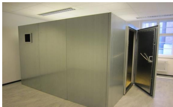
Faraday Cage used to test RF emissions.
